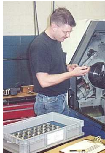
Jeff (TMC), inspecting and packing KANBAN bin. No looking for packing material, precision parts protected and the empty bins trigger the next production run.
